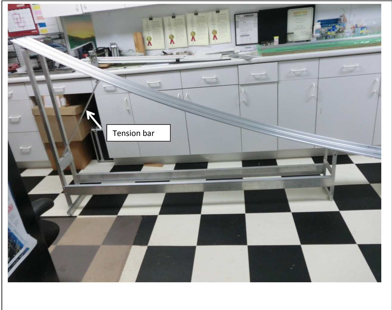
Figure 3 – Showing the tension bar used to curve track at the “sweet spot” described in the text
