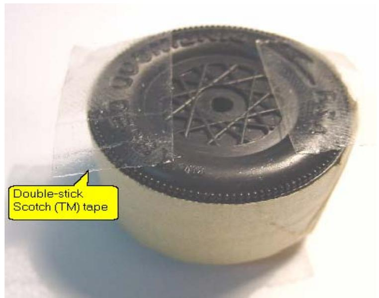
**Figure 4** - Put double-stick tape on the drill bit guide.
