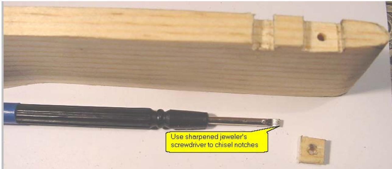
Figure 22 - Mark notch edges on sides of car.
