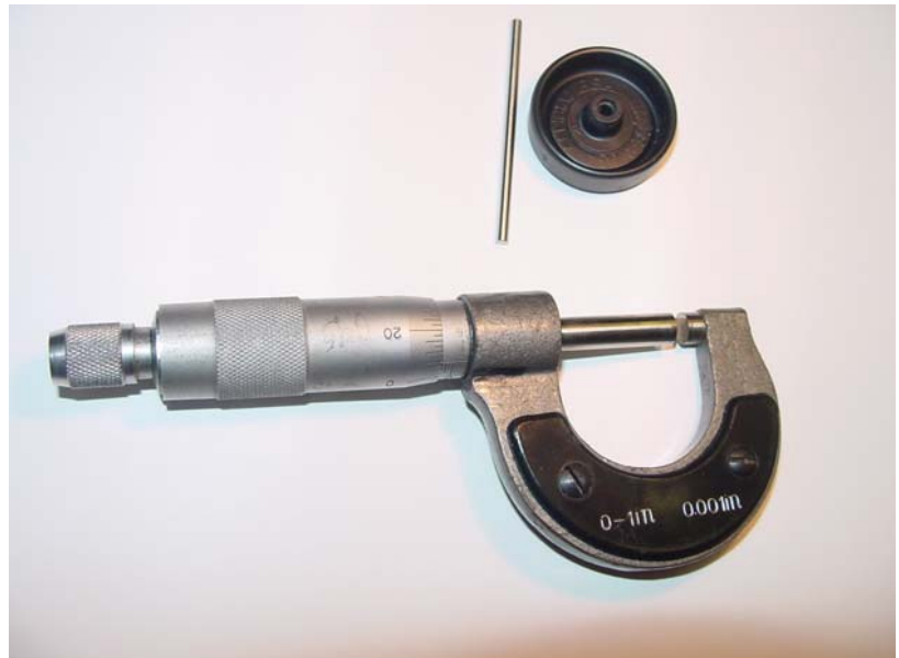
Figure 1. Micrometer calipers with a constant torque clutch next to a pin gauge of 0.1000" diameter used to calibrate the calipers for measuring drill bit shafts.
